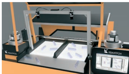
PET Preform Online Quality Control Inspection Machine
